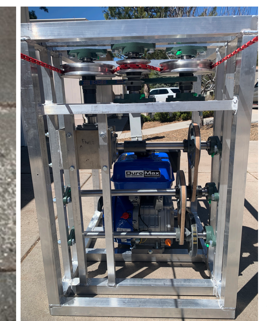
Figure 12: Final manufactured drive unit
